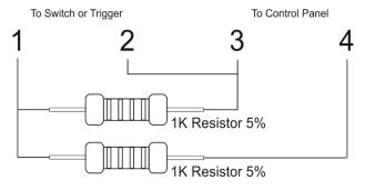
Normal Resistance: 2K  $\Omega$ ; Alarm Resistance: 1K  $\Omega$  Shorted Resistance: 0  $\Omega$ ; Open Resistance: Infinite  $\Omega$
